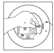
a. Turn the thumbscrew and open the hinged door located inside the back box.
